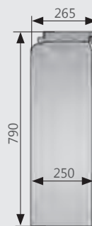
Narrow side panel – NS (weight: 1.7 kg)
