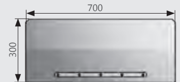
Narrow upper shields - side, 2x each (weight: 0.6 kg / 0.8 kg)
