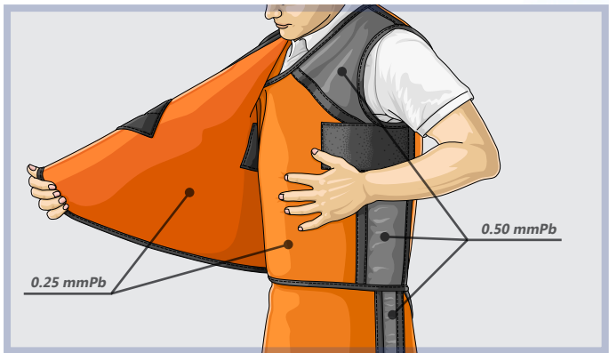
Fig. 6: Colour-contrasting safety zones to ensure that the vest and skirt are securely closed. In this example, the costume has a lead equivalent value of 0.50 mmPb.
